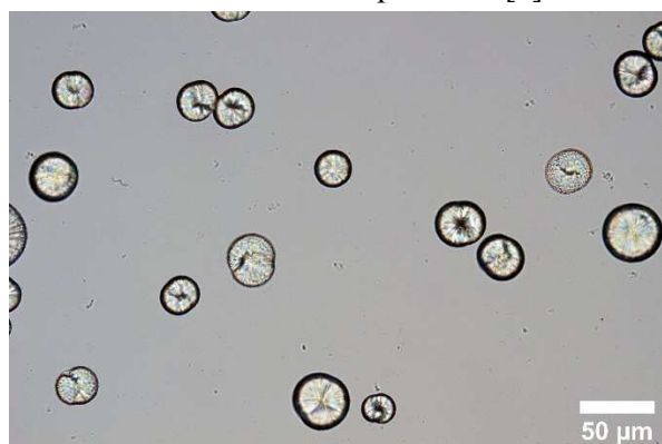
Fig. 1 Microparticles formed from 10 mg·mL -1 of P1 and 1 mg·mL -1 of Dexa in distilled water examined by optical microscopy with visible light at temperature 40°C.
